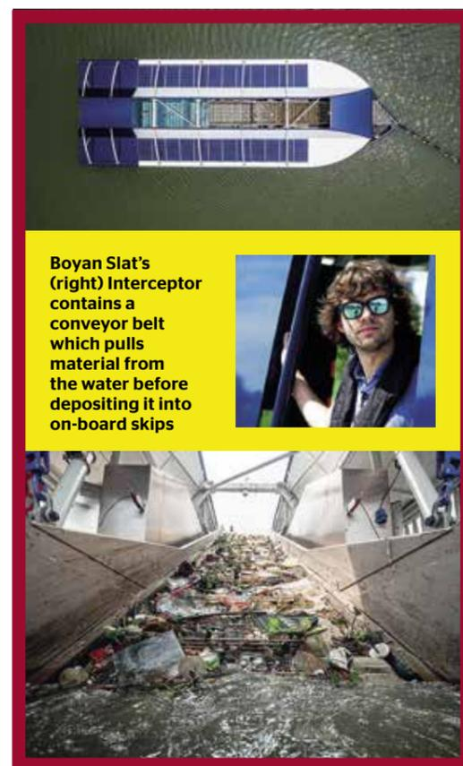
Boyan Slat's (right) Interceptor contains a conveyor belt which pulls material from the water before depositing it into on-board skips
